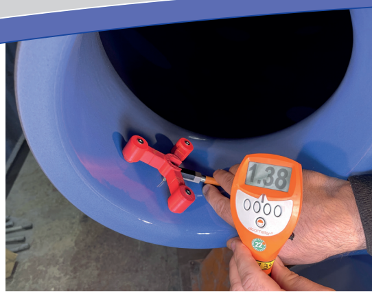
② 2: Schichtdickenmessung an einem RefPoint Layer thickness measurement on at a RefPoint
